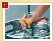
Place tap body into opening at top of barrel. Turn tap body clockwise until it is firmly in place.
