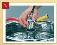
Place tap body into opening at top of barrel.
